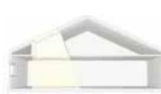
If you have an upstairs or single-storey room with a flat ceiling, you can construct a light shaft to cut through the loft and let light into the room below.
