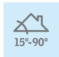
Suitable for roof pitches between 15° and 90°.
