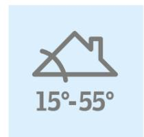
Suitable for roof pitches between 15° and 55°. Also suitable for roof pitches between 55° and 75° with special springs – please specify when ordering.
